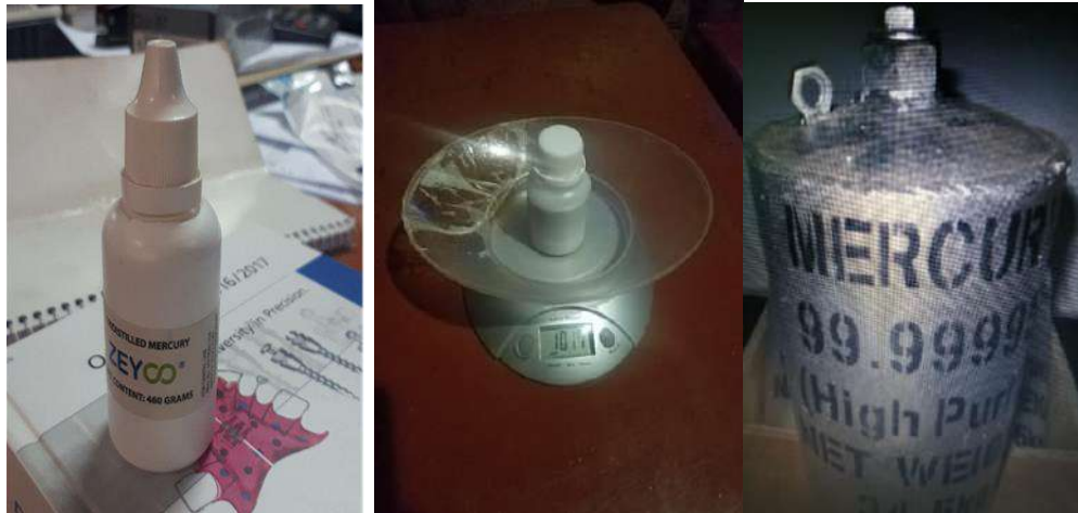
Figure 4-2: Dental amalgam (460 g), Hg in plastic container (1 kg) and Hg in metallic cylinder (34.5 kgs) respectively.
