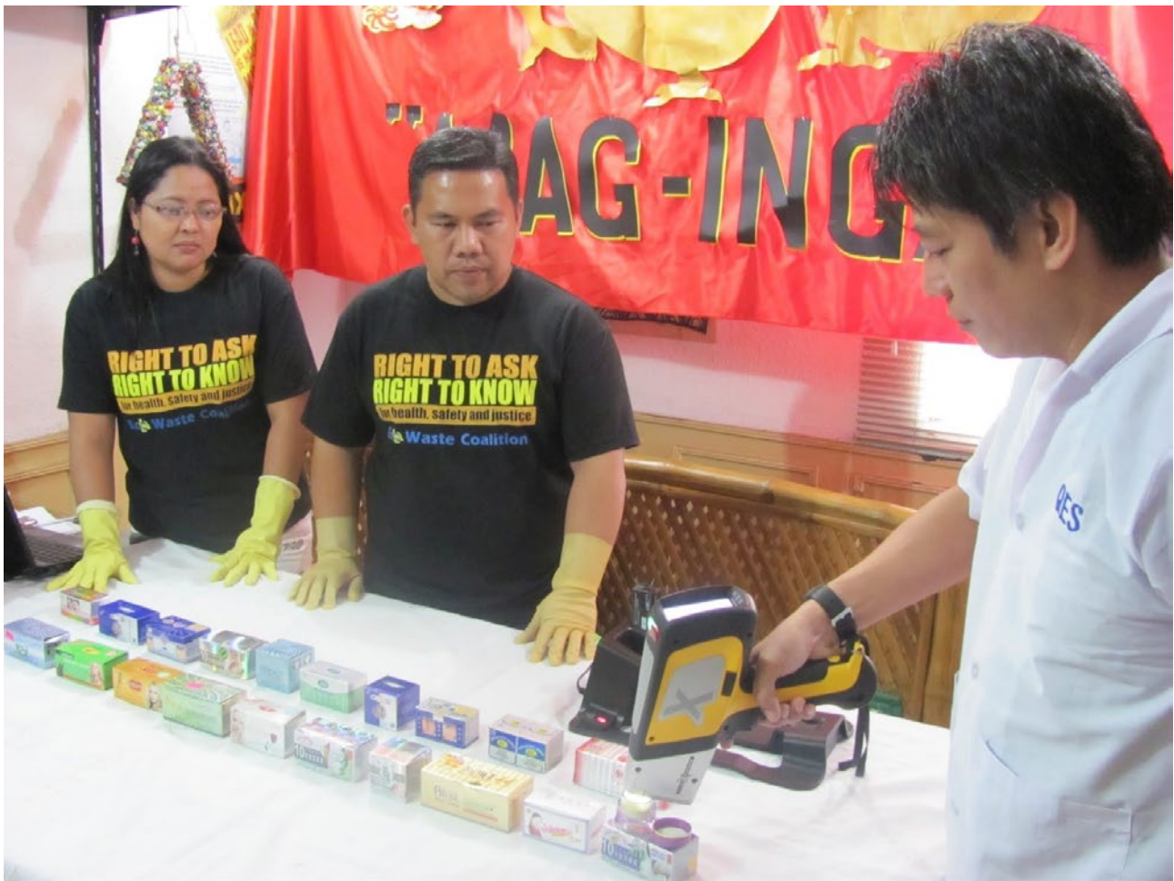
Photo 8: EcoWaste Coalition, a participating organization of IPEN, successfully using a handheld XRF for analysis a large variety of products for total bromine and antimony levels, proxies of PBDE content in products. Photo: EcoWaste Coalition.
